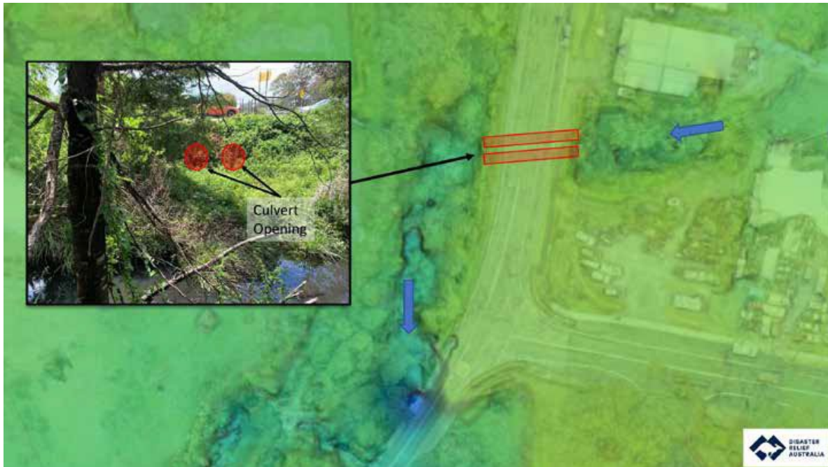
Image 10: 2 culverts 0.9m in diameter allow water to drain from the business centre to the east to Cabbage Tree Creek on the western side of the highway. Culverts we identified in the TMPBM Flood Study 2017 as inadequate in diameter.
